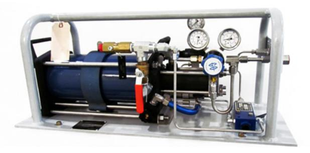
Most hydraulic accumulators need to be precharged with dry nitrogen gas before operation. Accumulators, Inc. nitrogen gas boosters are designed to boost gas pressure directly from nitrogen cylinders to outlet pressures as high as 10000 psi. Our unit ensures maximum outlet pressure will be maintained even if the pressure in the nitrogen cylinders drops as low as 500 psi.
